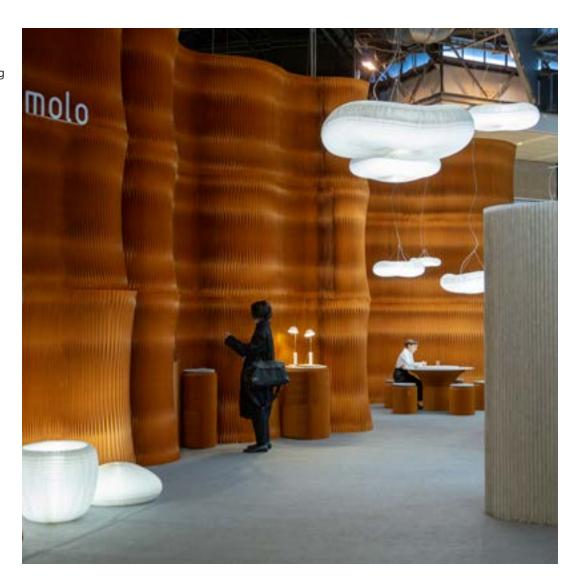
The hollow cloud shades, made from white polyethylene non-woven textile, are internally lit by LEDs, making the sculptural three dimensional forms mysteriously radiant when viewed from any direction, with no visible hot spots.
