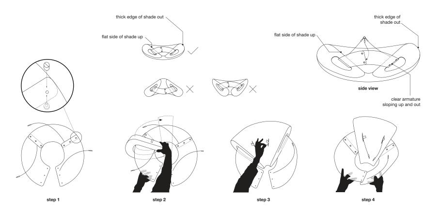
step 1: To assemble the cloud armature, peel off protective paper and lay all three clear plastic pieces on a flat surface. Check that the crimped loop-end of each steel support cable is on the top side. Hand-turn the chicago bolts to unscrew, and then line up holes of armature as shown above. Ensure that the side with attached support cable is underneath the piece to be connected. Screw pieces together to create a "C" shaped collar. Do not close the collar
