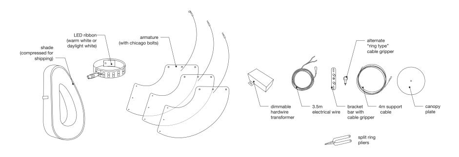
dimmable hardwire transformer: Dimensions and watts vary with cloud size, as shown on right. 120V and 240V options available. Mount transformer behind electrical junction box in ceiling or other accessible location. Specifications can be found inside the transformer box. Dimmable with standard magnetic low-voltage (MLV) dimmers. - small cloud pendant:
