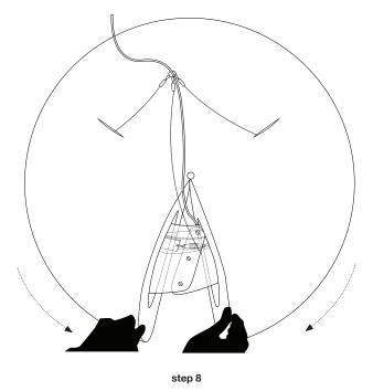
**step 8:** Close the shade around the armature by holding inside the shade cavity and pulling the magnetic end panels around, connecting to each other. The magnets hold the end panels together. The third steel support cable and electrical wire sandwich between the two magnetic end panels.
