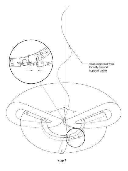
**step 7:** Connect electrical wire to LED (be sure to line up matching groove in male and female ends of connectors).
