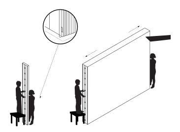
With person 1 stationary and firmly holding softwall, person 2 begins to pull open softwall, first expanding the columns of honeycomb cells nearest the end panel and then continuing with each adjacent layer. While opening, lift lower end of softwall 3 centimeters (1 inch) off the floor, rather than dragging it. Once the first 20-30 layers have expanded, continue opening softwall to its full length. Hold softwall in this expanded position for a few minutes to stretch
