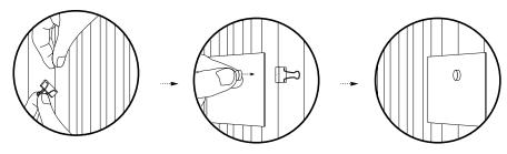
step 1: Attach a steel clip to a vertical fin.
