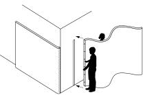
An acoustic wall liner can be made by magnetically connecting thinwall to molo steel strips.
