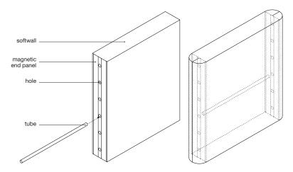
configuration - arrangements of tubes The point where two tubes meet can become a hinge to create angular configurations.
