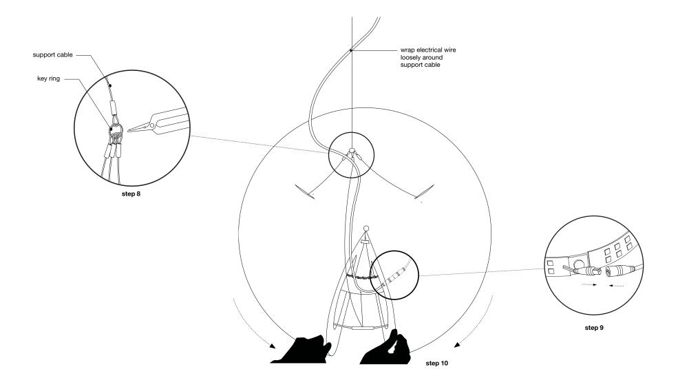
**step 8:** Use split ring pliers to open the key ring attached to main support cable and attach the three support cables from cloud pendant.
