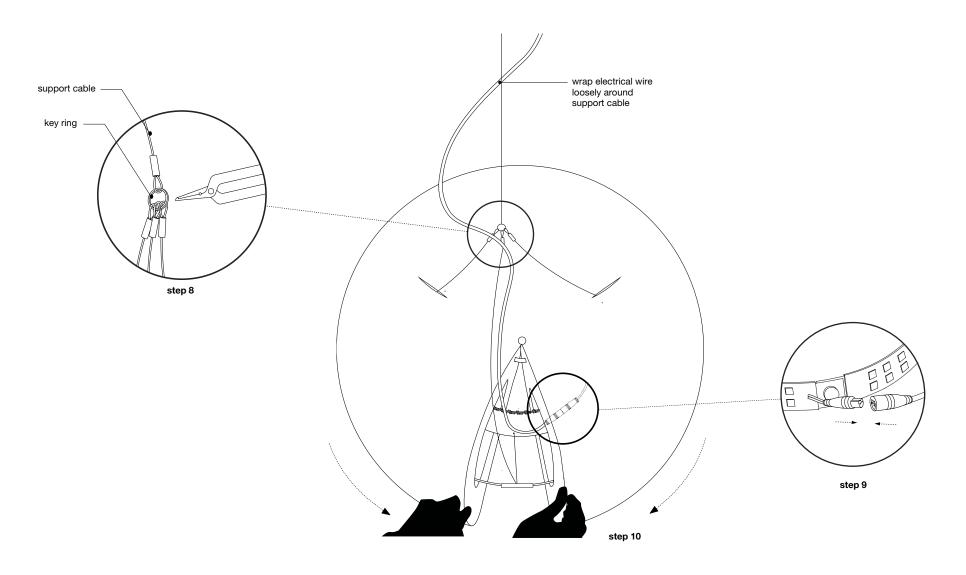
**step 8:** Use split ring pliers to open the key ring attached to main support cable and attach the three support cables from cloud pendant.
