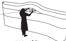
peg + strip reinforce the connection between horizontal layers of softblocks
