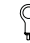
alternate "ring type" cable gripper (flexible option of hanging cloud pendants from wall hooks)
